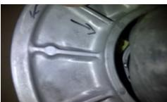
**Installing and winding of secondary sheave/spring** The spring must be engaged in the proper holes first, then carefully look at the splines. There is a master spline that must be aligned on the shaft and helix.
