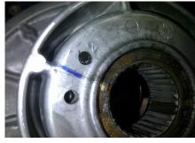
For this application, the secondary clutch spring will be remaining at **the factory setting of 2-2** in the torsional spring hook positions. (#2 hole in helix and #2 hole down in the clutch).
